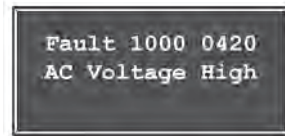
Figure 5-3 AC Voltage High/DC Voltage Low Fault
